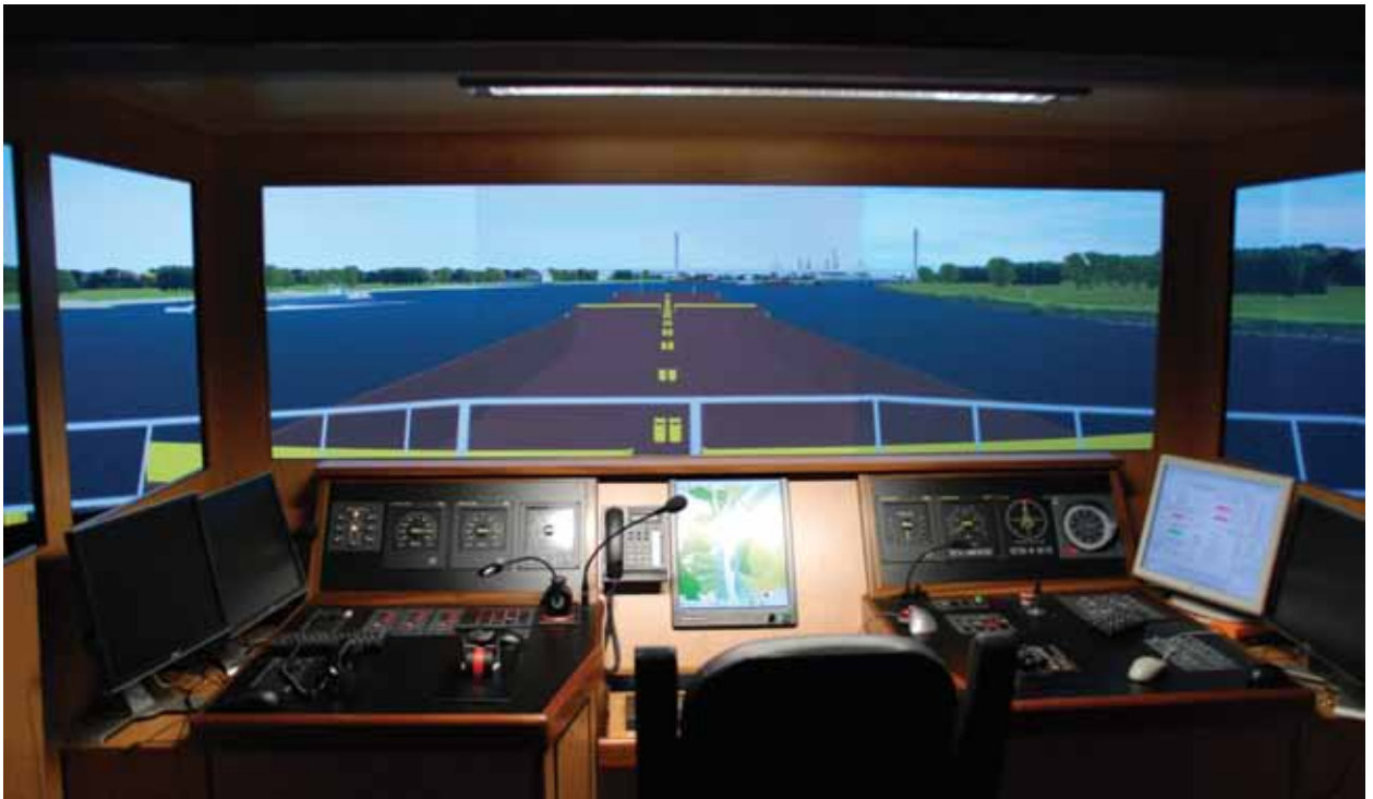
“SANDRA” shallow-water navigation simulator
