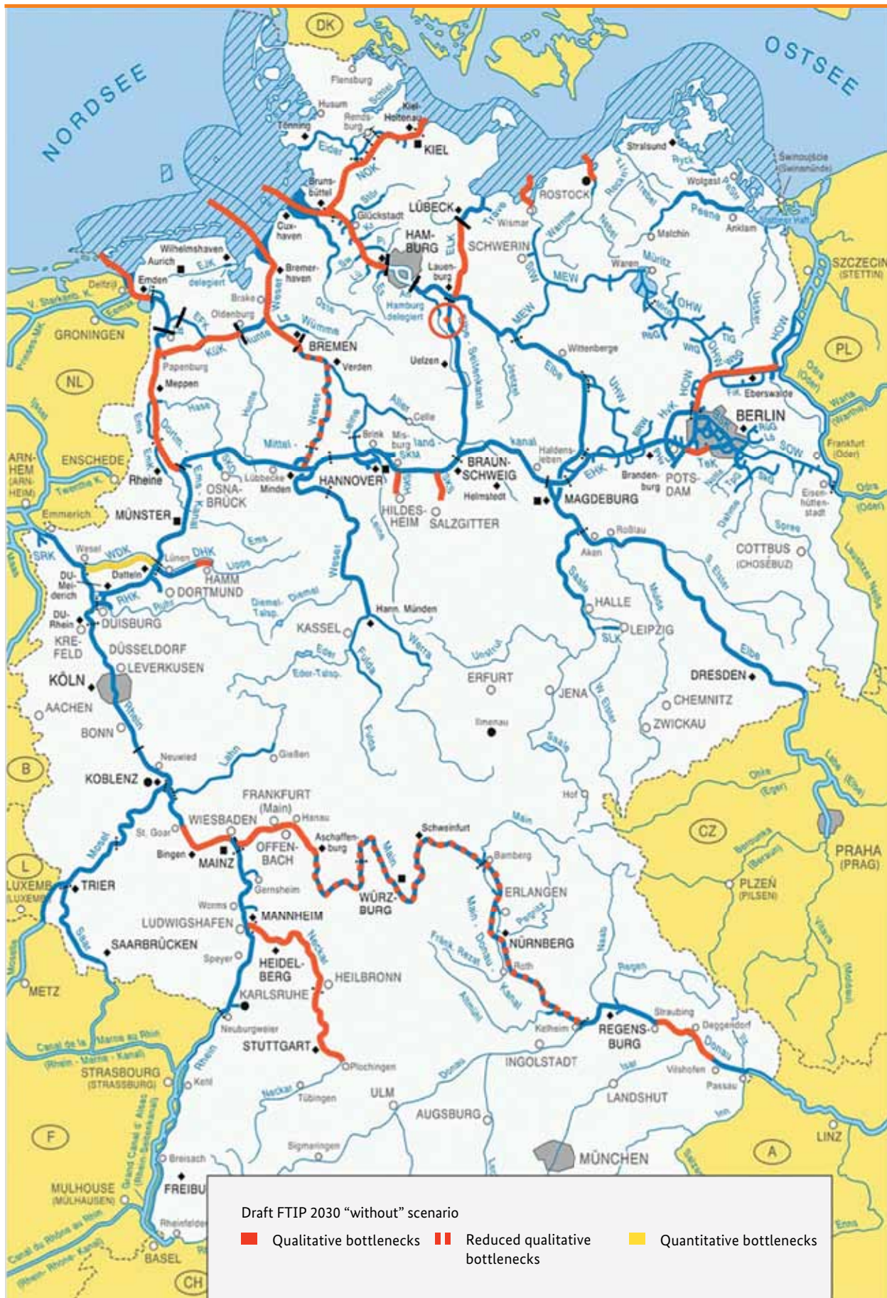
Figure 9: Analysis of bottlenecks on the waterways – “without” scenario
