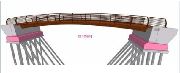
Figure 2: Example of model-based quantity take-off for pile caps for the bill of quantities (source: LSBG)
