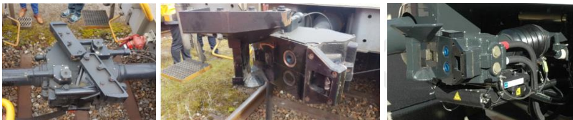
Fig. 22: Schwab couplings: RFT version in the 2018 “5L” demonstrator in MuttENZ, in coupled (left) and uncoupled states (centre), as well as in the mainline version (right)
