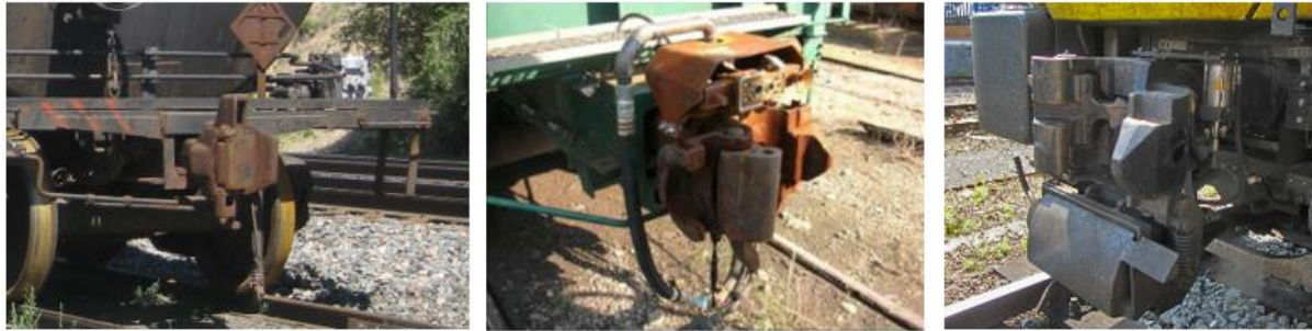
Fig. 13: Janney coupling with buffer override protection (left), fully automatic Type F (middle) and Buckeye coupling from England (right)
