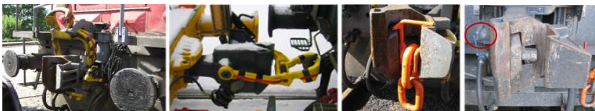
Fig. 6: From left to right: SA3 coupling with shunting adapter for SC folded up and engaged in the draw hook of the SC, “SA3” with attached SC adapter and “SA3” with additional horn (circled in red) on the left side for attaching the SC as a draw hook replacement.
