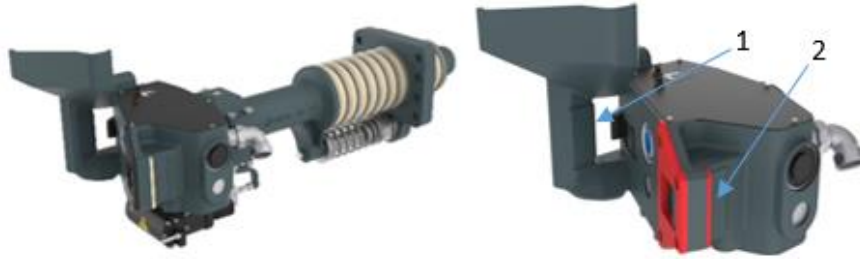
Fig. 24: DAC Type 4 Schwab coupling (left), Schwab head with wear plates marked in red (right)
