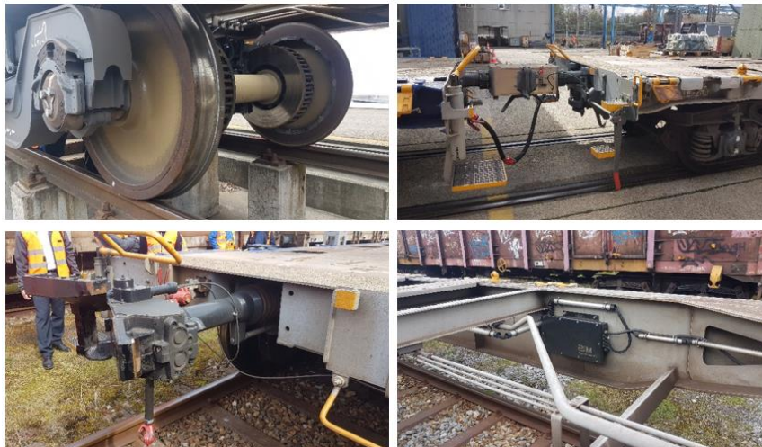
Fig. 42: Innovations in the 5L demonstrator: disc brake and wheel noise absorber (top left), Voith AC (top right), Faiveley AC (bottom left) and sensor technology (bottom right)
