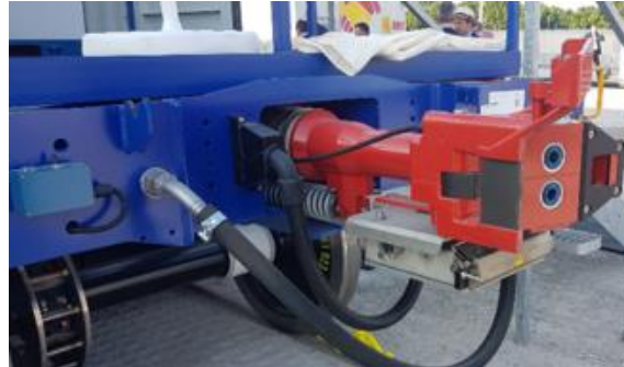
Fig. 25: Prototype DAC Type 4, “Type 5 - Ready” exhibited at the transport logistic trade fair in Munich in 2019
