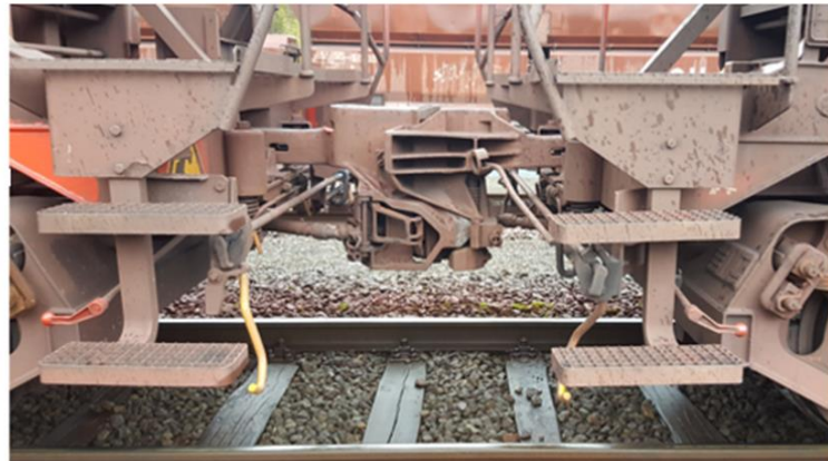
Fig. 36: Operating controls in accordance with UIC MB 535-2 incl. positions (left), coupled “AK69” with clearly visible operating control (yellow) in the basic position as well as separately available end cocks with red handles (right)
