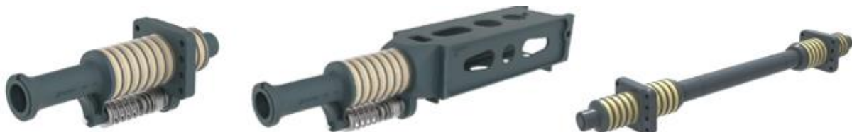
Fig. 31: Horizontal suspension of Schwab DAC without (left) and with UIC insert (centre), derived from a conventional, rigid, fixed freight wagon coupling (right)
