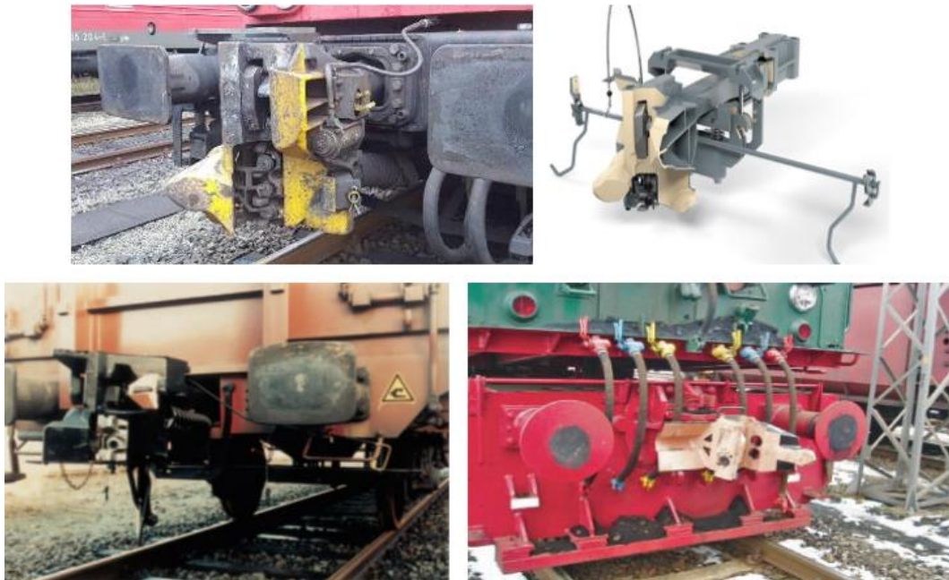
Fig. 15: “AK69” (top left), “Modular SA3” from Voith (top right), “Z-AK” (bottom left), “C-AKv” (bottom right)
