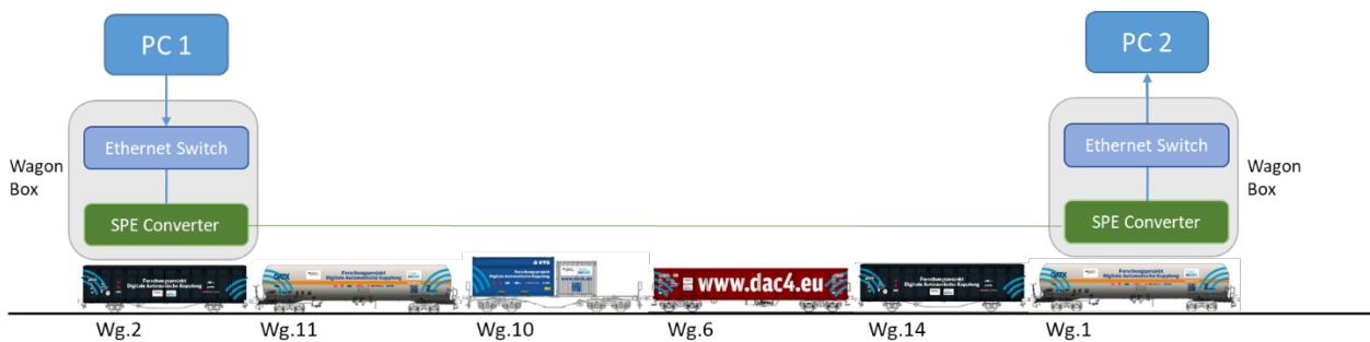
Figure 11: SPE communication test via a continuous line
