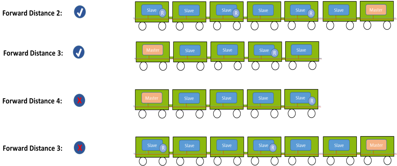
Figure 12: Test of the Powerline-PLUS forward distance in a wagon-set
